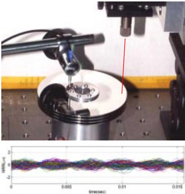
**Figure 8. Testing of encapsulated spindle design with aluminum baseplate for NRR at 10 KRPM.**
