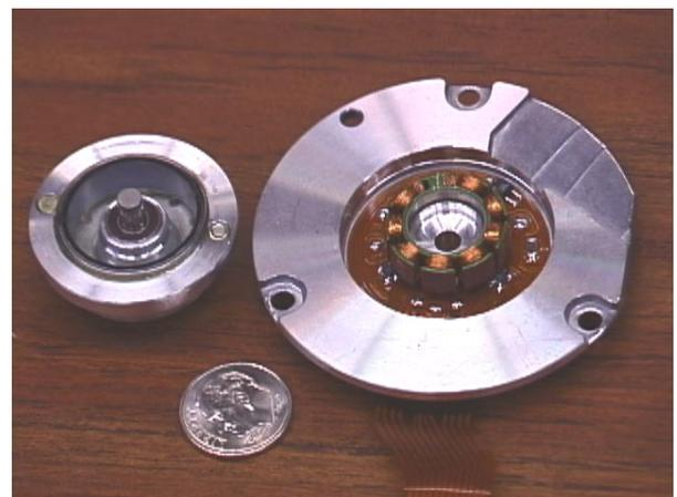
**Figure 1. Conventional disk drive spindle motor**
