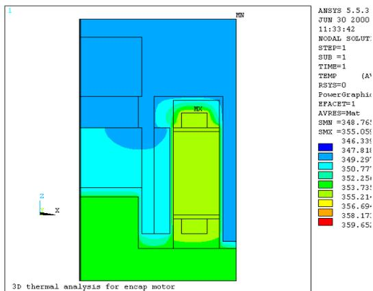
**Figure 5. Temperature when thermoplastic encapsulation of k=1**
