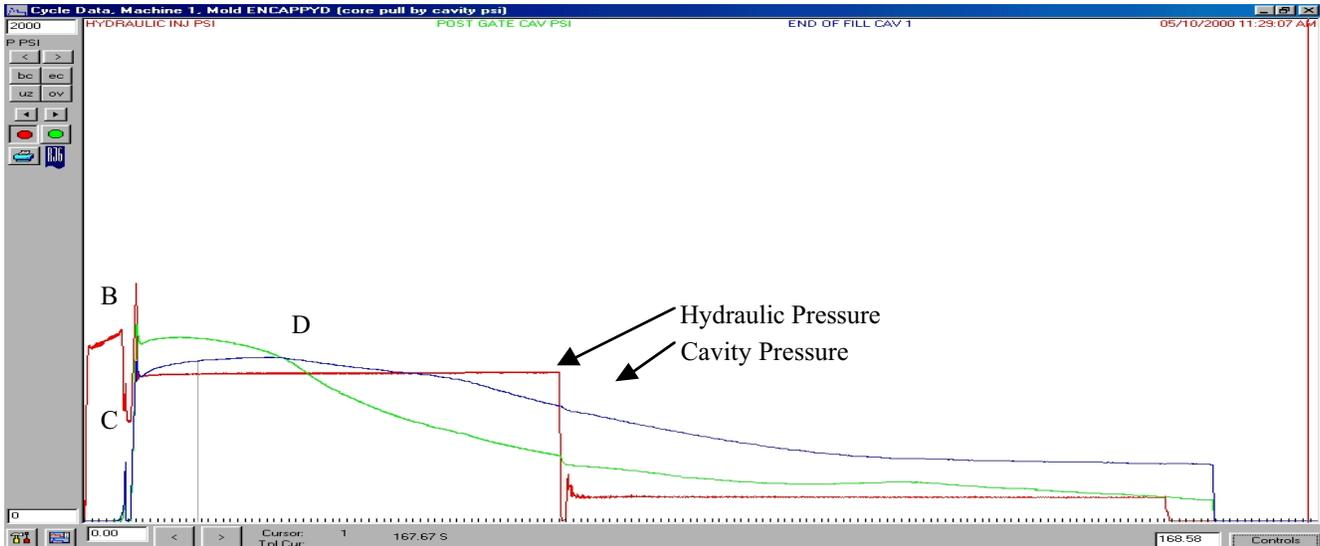
**Figure 10. Process pressures for encapsulated ROV stator (time vs pressure)**
