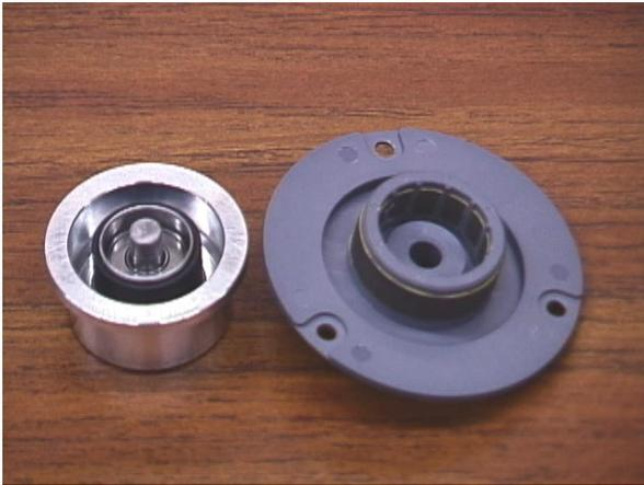
**Figure 2. Unitized stator/baseplate assembly**
