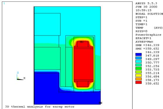
**Figure 4. Predicted coil temperature when encapsulation is not used**
