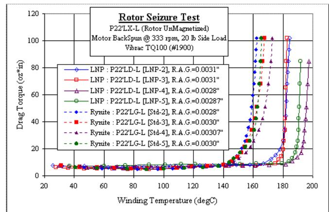
**Figure 3. Rotor seizure comparison**
